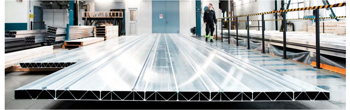
Extrusions are often cut and joined
